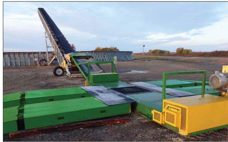
Tazz Corn Hog drive-over conveyor (lower right) delivers corn to a 15,000-bph Allatoona radial stacker. Photo courtesy of MaxYield Cooperative, West Bend, IA.
